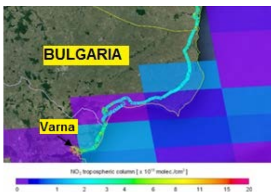
Figure 7. Mobile DOAS measurements and OMI observations on 19 May 2016, in Bulgaria
