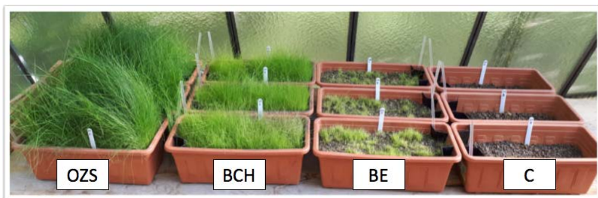
Figure 2. Pot experiment with soils from Libiola 12 weeks after its establishment (OZS – technosol + organo-zeolitic substrate, BCH – technosol + biochar, BE – technosol + bentonite, C – control sample)
