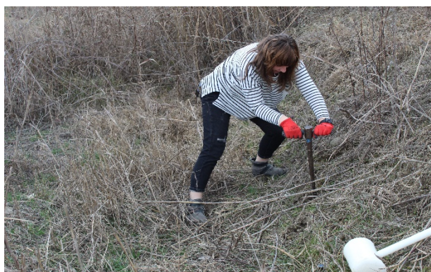
Figure 5. Sampling with Augher method.
