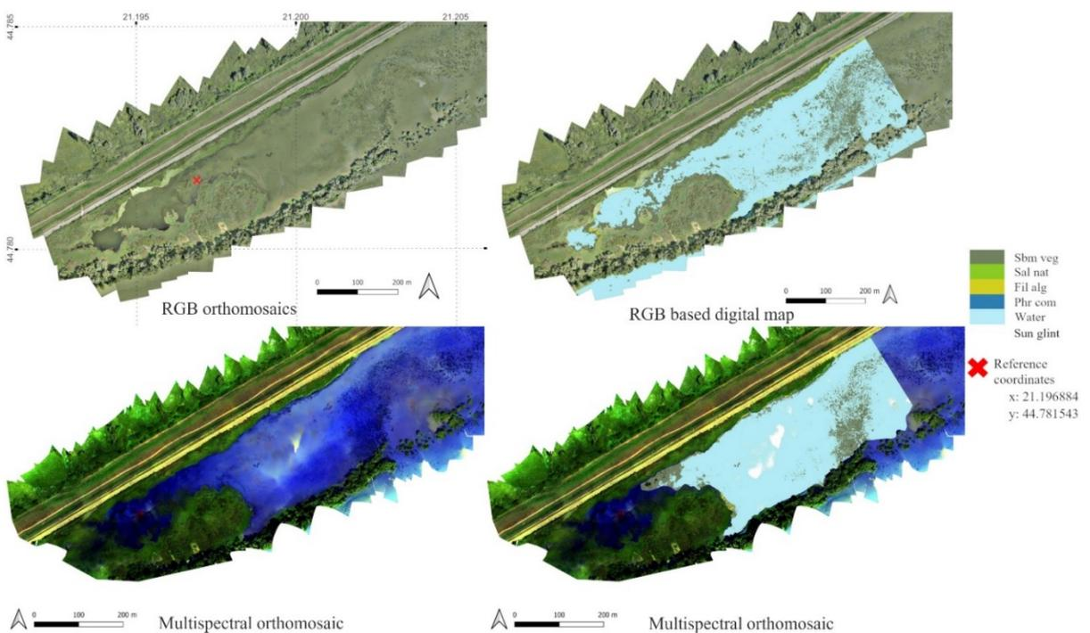
Figure 4. Orthomosaics and digital maps of the Dubovac (A) river section
