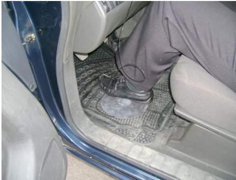
a) Triaxial accelerometer (SEAT) under the foot
