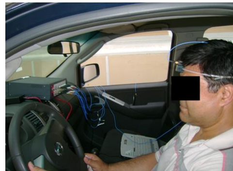
d) Triaxial accelerometer on the forehead
