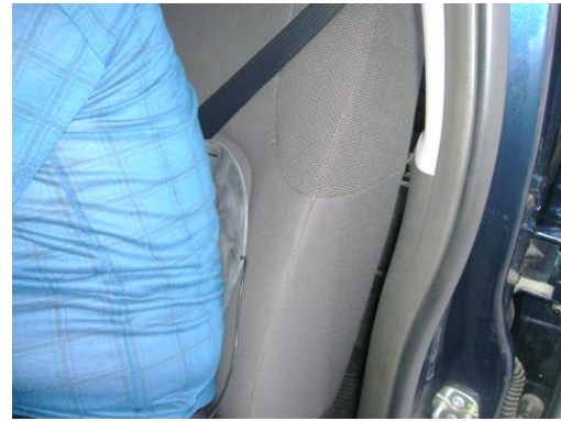
b) Triaxial accelerometer (SEAT) on the lumbar
