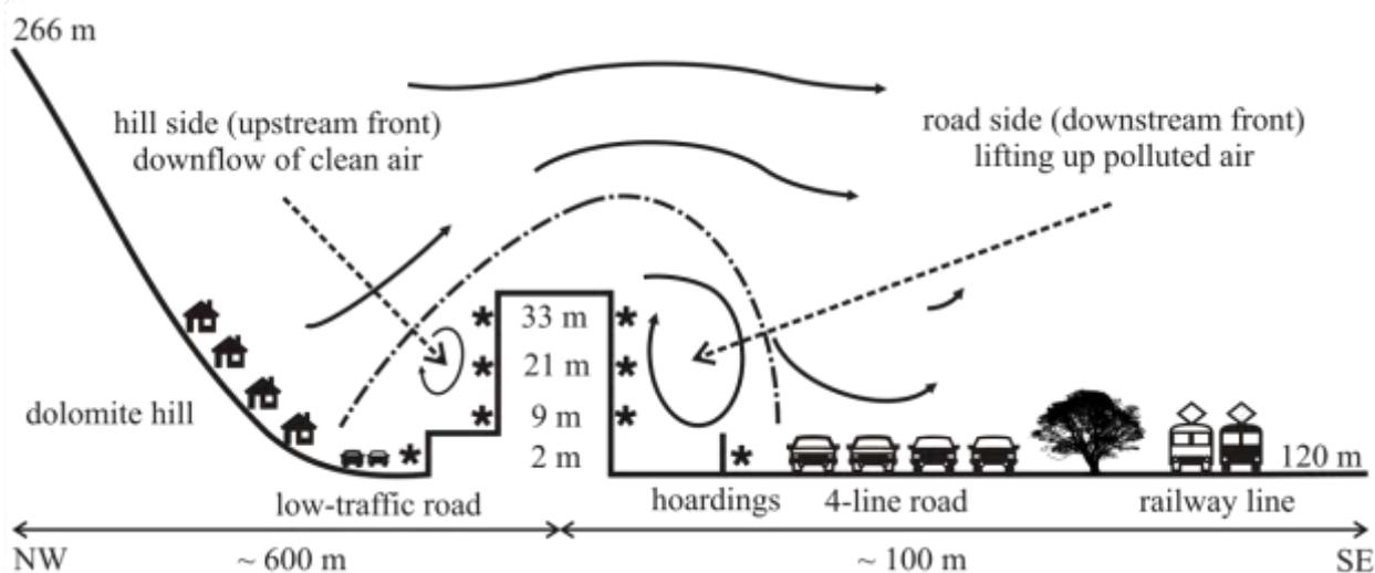
Figure 1. Sketch of the surroundings of the sampling site showing the isolated roughness air-flow model. Sampling locations are shown by the stars (\*), supposed air-flow directions by continuous arrows.
