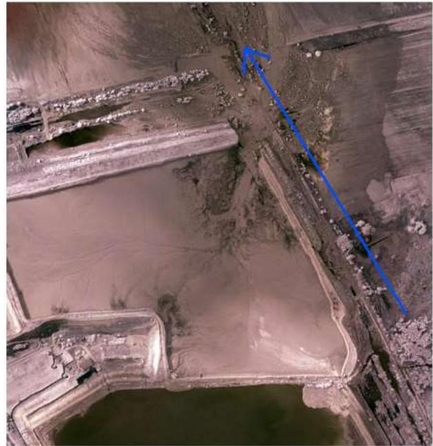
Figure 5. Signs of wetness near the northern dam section in NIR air-shot /with the arrow showing the direction of slope/
