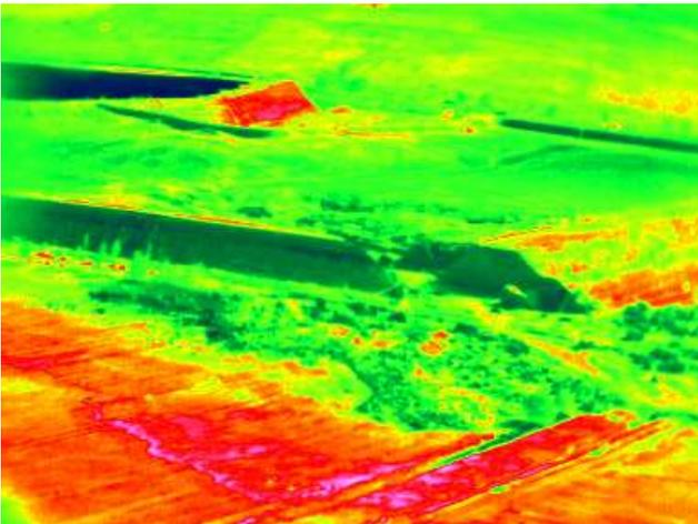
Figure 4. Identification of wet and dry areas near the reservoir in lateral's thermo-shot (warmer condition because of dryer surface - red in bottom, cooler condition because of flowing off - dark green in bottom).
