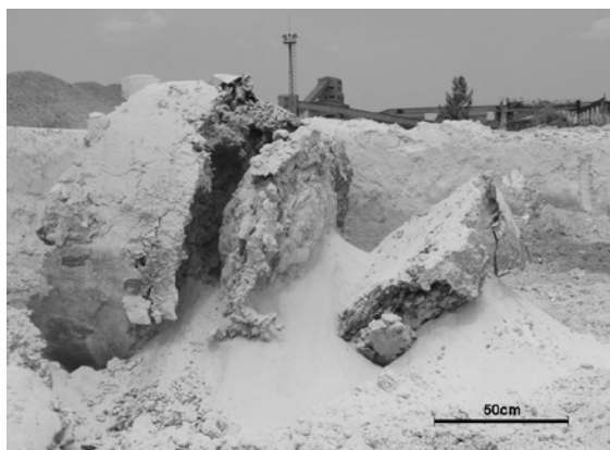
Figure 1. Disintegrated secondary slag in the slag heap of OAM Ltd.
