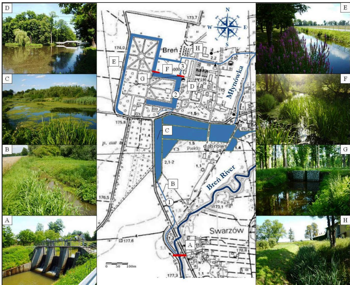
Figure 2. Location of measurement-control points and other elements of the irrigation system Explanations: 1, 2 and 3 – location of the measurement-control points; A – three-span flap weir on the Breń River; B – the supply ditch; C – ponds; D – the main channel in the manor-park complex with a white bridge; E – the West channel; F – the North channel; G – two weirs to damming up of the water; H – the discharge ditch.
