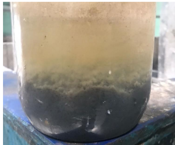
Figure 3. Ballast water sludge deposits after the sedimentation process.
