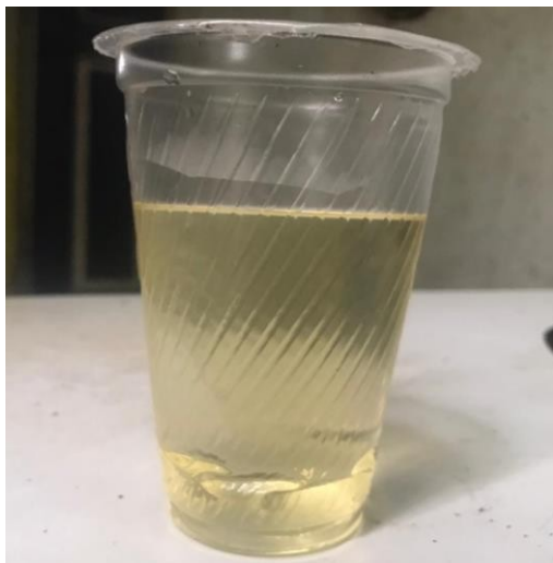
Figure 4. Ballast water after the electrocoagulation and filtering process
