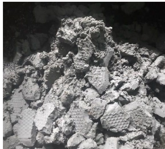
Figure 5. Sludge or ballast water residual cake in the filter press tank.
