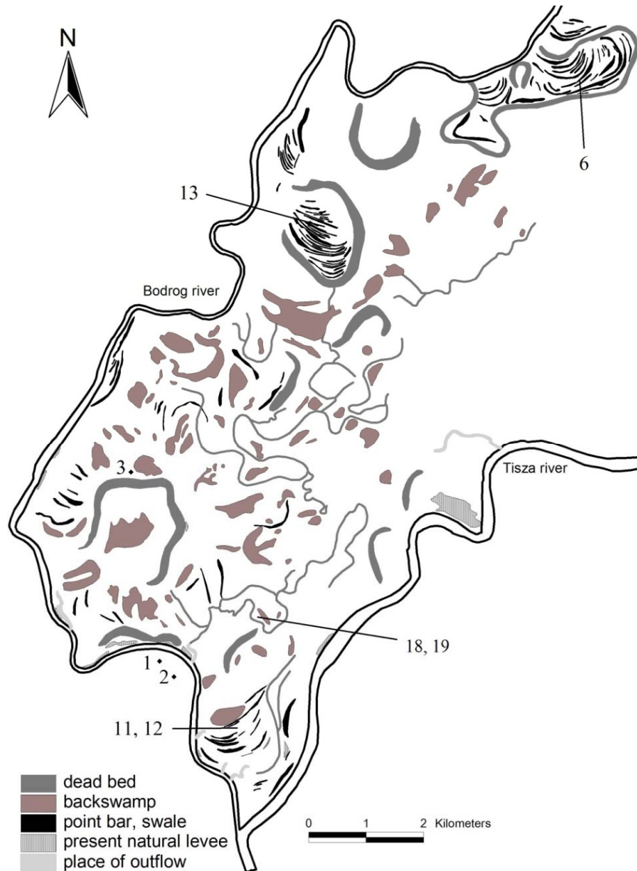
Figure 9. Geomorphological map of Bodrogzug. The numbers show the place of sediment traps.
