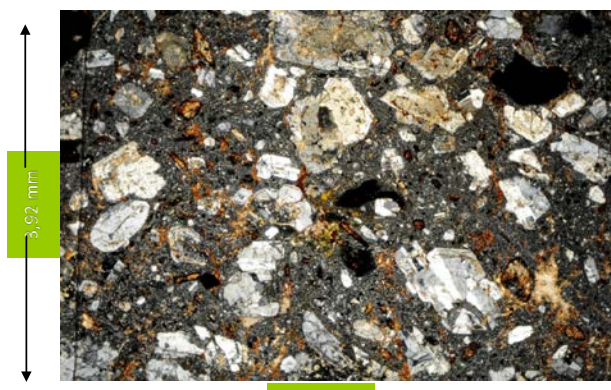
Partial substitution of the internal zones of plagioclase feldspar. There is a lot of siderite-ankerite grains, and also idiomorph prismatic oxihornblende, partly opacitized, into the microcrystalline fundamental mass. N+
